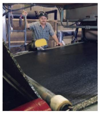
Vitafoam's Maintenance Supervisor Dave Matthews checks the quality of the foam lamination. Using Paratherm LC™ system cleaner, Vitafoam eliminated the cold spots on the rollers that were caused by fouling.
